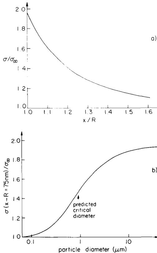
Fig. 6. (a) The stress enhancement in the glassy matrix outside the particle on its equatorial plane as a function of normalized distance from the particle center.  $x$  is the distance from the particle center, and  $R$  is the particle radius. (b) The stress enhancement at a distance 3 fibril spacings (75 nm) from the particle interface vs. particle diameter.
