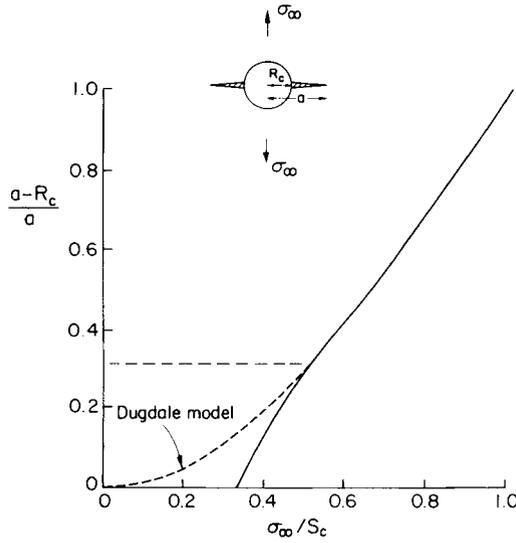
Fig. 2. Predicted length  $a$  of a thin yielded zone with constant yield stress  $S_c$  growing from a cylindrical void of radius  $R_c$  in a thin sheet under an applied stress  $\sigma_\infty$  [after Tada et al.<sup>20</sup>]. The dashed line shows the predictions of the Dugdale model where the zone is assumed to grow from a planar crack of half-length  $R_c$ .
